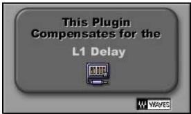
Delays the signal by 64 samples to compensate for the lookahead in L1UltraMaximizer as well as Renaissance Compressor, Renaissance VOX and L2UltraMaximizer.
